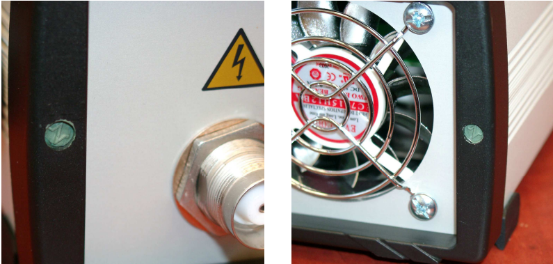
Fig.6. Warranty seals at the front and rear panels.
