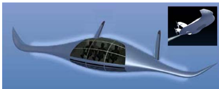
Figure 1. Hybrid flying wing with two 260 kW all-electric engines and distributed plasma jet propulsion.
