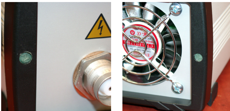
Fig.14. Warranty seals at the front and rear panels.
