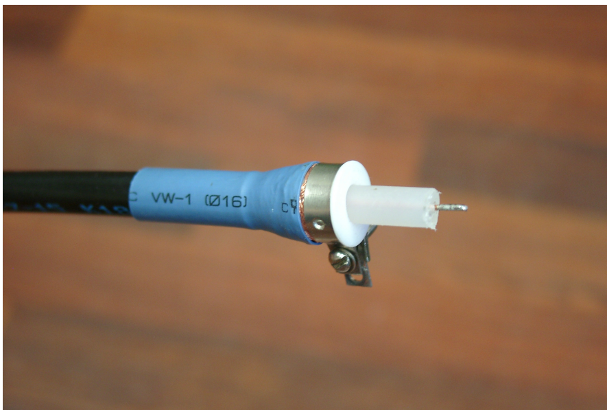
Fig.2. Teflon cone insulator on the cable end.
