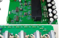
by Jumpers and therefore deactivated. This allows to reduce the transformer ratio of nominal 1:184 to 1:158, 1:132, 1:106 and therefore to drive higher capacitive loads respective lower impedances with however lower output voltages.
